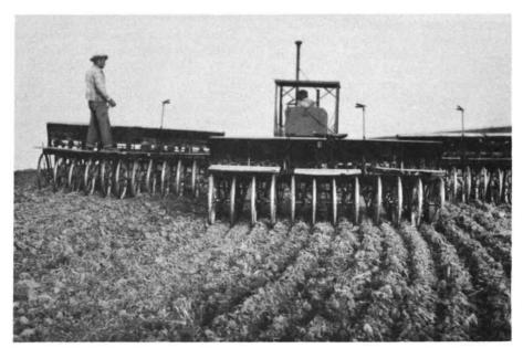
Figure 5.—Gang drills with large packer wheels are frequently used for sowing oats on the dry lands of the Great Plains area. (Courtesy of the Fort Hays Branch Experiment Station, Hays, Kans.)
