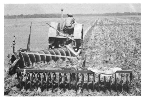
Figure 2.—Preparing a seedbed for oats with a one-way plow and packer in western Kansas. (Courtesy of the Fort Hays Branch Experiment Station, Hays, Kans.)
